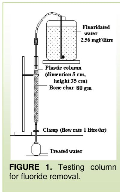
**FIGURE 1.** Testing column for fluoride removal.
