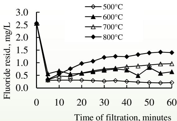
**FIGURE 2.** Average residual fluoride concentration after filtration by calcined bone char at different temperatures (bone char 80 g, flow rate 1 L/h,  $S_0=2.56$  mg F/L)
