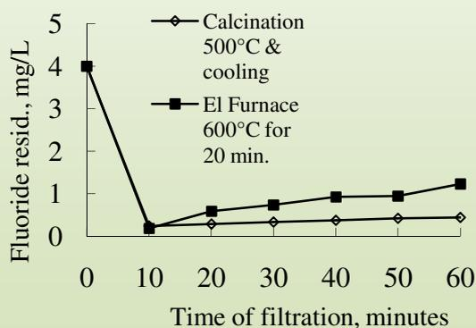
**FIGURE 3.** Average residual fluoride after filtration by calcined and pyrolysed bone char.
