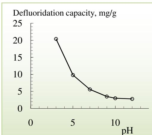
**FIGURE 1.** Defluoridation capacity of activated alumina at various pH values of the environment
