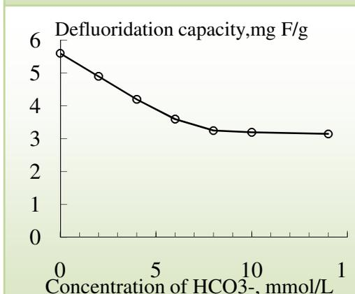
**FIGURE 2.** Defluoridation capacity of activated alumina at various concentration of bicarbonate ion.
