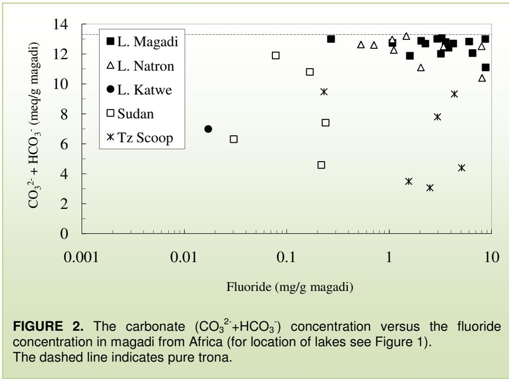
**FIGURE 2.** The carbonate ( $\text{CO}_3^{2-} + \text{HCO}_3^-$ ) concentration versus the fluoride concentration in magadi from Africa (for location of lakes see Figure 1). The dashed line indicates pure trona.
