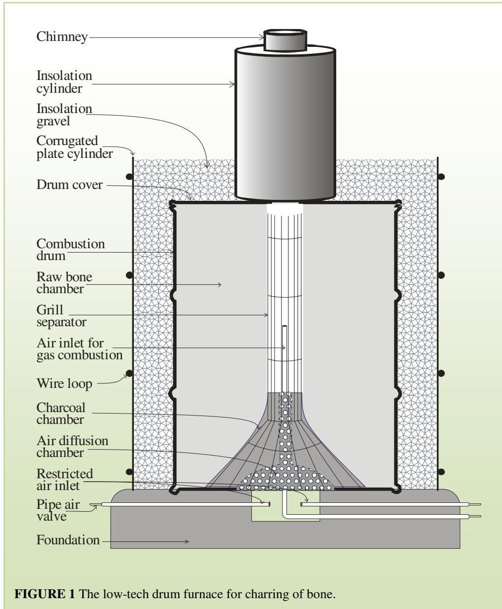
**FIGURE 1** The low-tech drum furnace for charring of bone.
