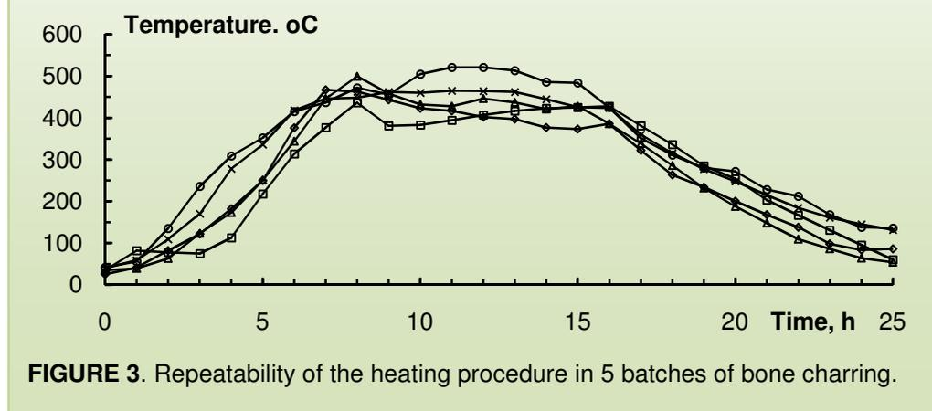
FIGURE 3. Repeatability of the heating procedure in 5 batches of bone charring.
