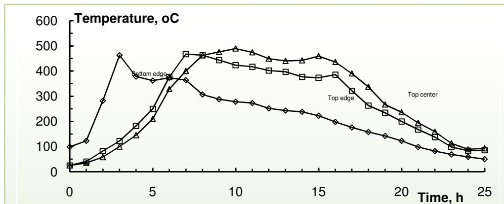
FIGURE 2. Monitoring of the temperature during a charring cycle in the furnace.
