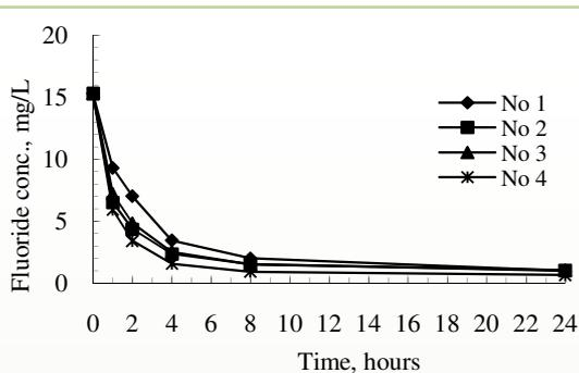
**FIGURE 1.** Defluoridation of water by the use of soil from the Ethiopian highland. The soil was heated at 250°C for three hours. The dosage was 10 g/L.
