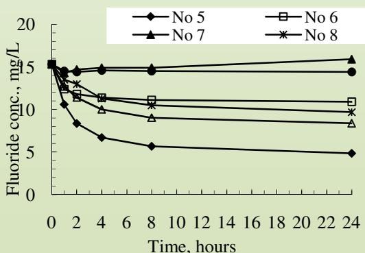
**FIGURE 3.** Defluoridation of water by the use of soil from the Ethiopian Rift Valley. Heated for three hours at 250°C. Dosage 100 g/L.
